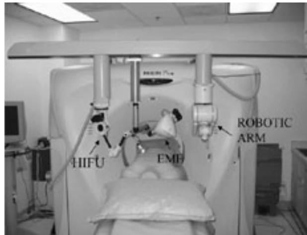
Fig.11 Prototype CT Scanner developed by the NIH and Philips Medical Systems incorporates tools that are mounted on a stereotactic frame : diagnostic US, high-frequency focused-ultrasound (left), EMF tracking (middle), robotic arm for precise "point-and-click" needle placement. This system allows for precise cross-registration of the spatial frame-of-reference of the patient (scanner) with that of the tool (Reprinted with permission from : Touring the Radiology Department of the Future. Health Imaging and IT 2005 ; August : 16-22 ; Courtesy : Brad Wood, MD (NIH) and Philips Medical Systems )
