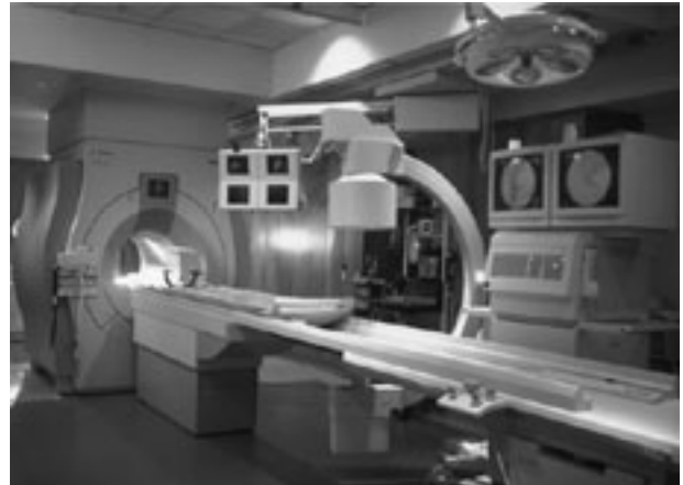
Fig.3 Philips XMR : A 1.5T MRI Scanner is installed co-axially with a digital subtraction angiography unit. The combination is beneficial for introducing and navigating catheters and guidewires under fluoroscopy while monitoring therapy with MRI. (Courtesy : Philips Medical Systems)
