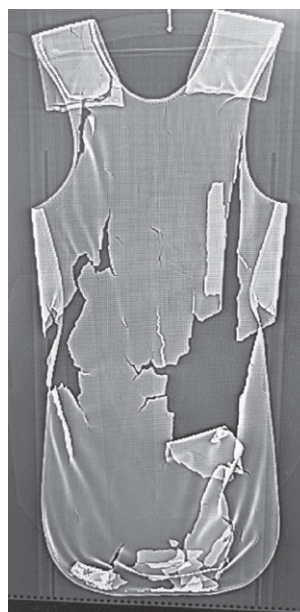
Fig.1 CT scanogram shows broken leaden sheet in the radiation protective gown.
